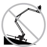
Do not raise the boom unless all four outriggers are lowered and locked, the footpads are in firm contact with the ground and the machine is level.
