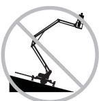
Do not raise or extend the boom unless the machine is level. Do not set the machine up on a surface where it cannot be leveled using only the leveling jacks. Do not use chocks, blocks or shims of any kind to level the machine.
