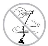
Do not operate the machine in strong or gusty winds. Do not increase the surface area of the platform or the load. Increasing the area exposed to the wind will decrease machine stability.
